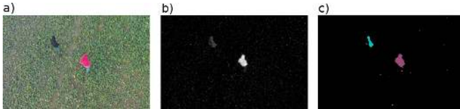
Fig. 6. a) input image, b) saliency map of the input image, c) ROIs extracted from the saliency map.
