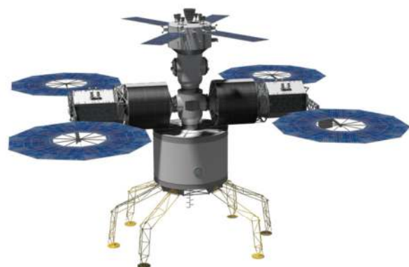
Figure 7 – Phobos surface habitat concept with top-mounted crew taxi and service module (Cases F and G).
