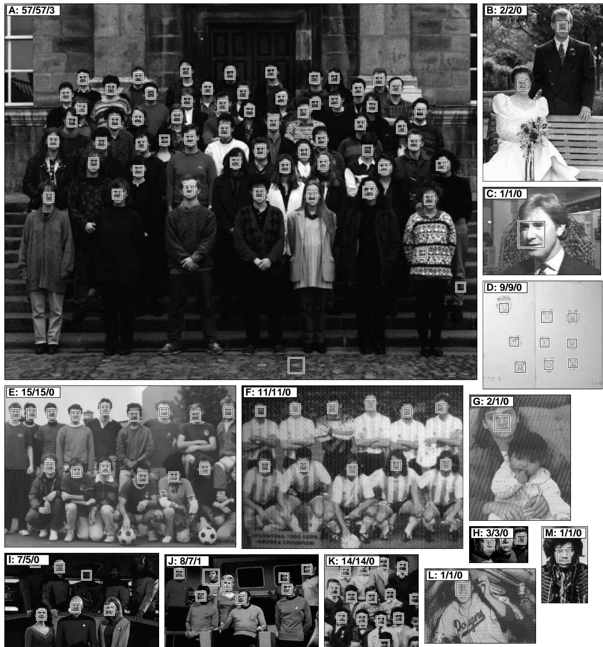
Figure 11: Output obtained from System 11 in Table 1. For each image, three numbers are shown: the number of faces in the image, the number of faces detected correctly, and the number of false detections. Some notes on specific images: False detections are present in A and J. Faces are missed in G (babies with fingers in their mouths are not well represented in the training set), I (one because of the lighting, causing one side of the face to contain no information, and one because of the bright band over the eyes), and J (removed because a false detect overlapped it). Although the system was trained only on real faces, hand drawn faces are detected in D. Images A, I, and K were obtained from the World Wide Web, B was scanned from a photograph, C is a digitized television image, D, E, F, H, and J were provided by Sung and Poggio at MIT, G and L were scanned from newspapers, and M was scanned from a printed photograph.
