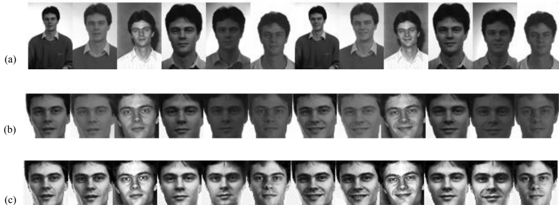
Figure 3.3: (a) Some samples from FERET database. (b) The result of the Viola-Jones face detection. (c) Images in (b) after histogram equalization.
