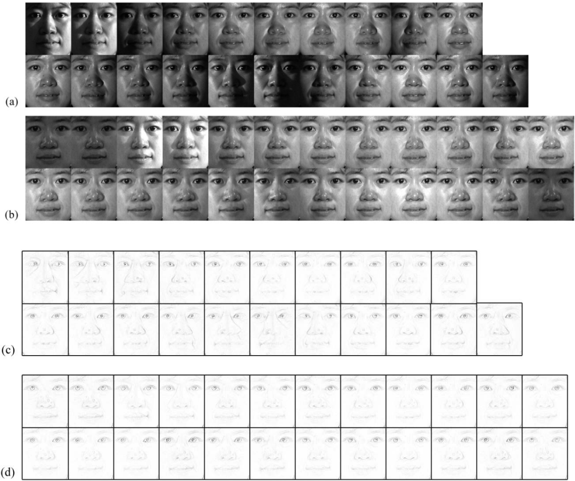
Figure 4.10: One of the samples in CMU-PIE database and its illumination invariants (a) lights-off group (b) lights-on group (c) and (d) are the corresponding illumination invariants to (a) and (b).
