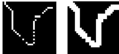
Figure 4.7: Edge enhancement property of the Maximum filter. The right image is the result of applying Maximum filter on the left image
