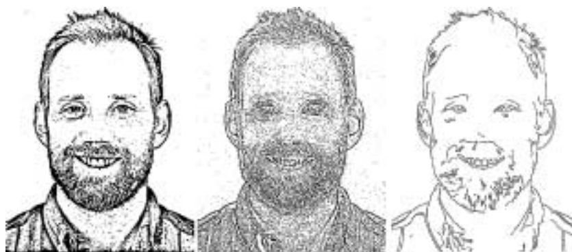
Fig. 3. Thresholded brightness (left), high-pass filtered image followed by thresholding (middle) and Canny's edge detector (right).
