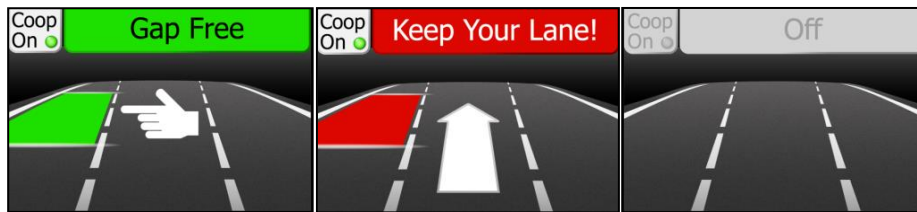
Figure 1. Sample pictures of the visual HMI: a) “lane change” recommendation; b) “keep your lane” warning; c) LCA inactive.
