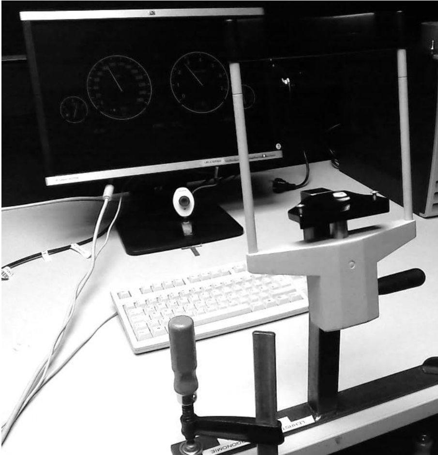
Figure 3 Setup of the occlusion task with a screen in front of the participants and a chin rest for the head.
