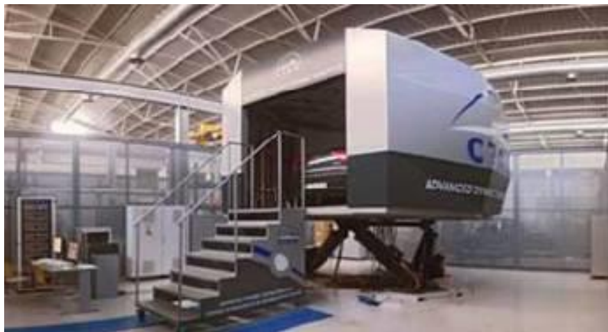
Figure 1. CTAG Dynamic Driving Simulator
