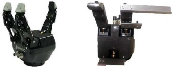
Figure 11. Robotiq finger modifications.
