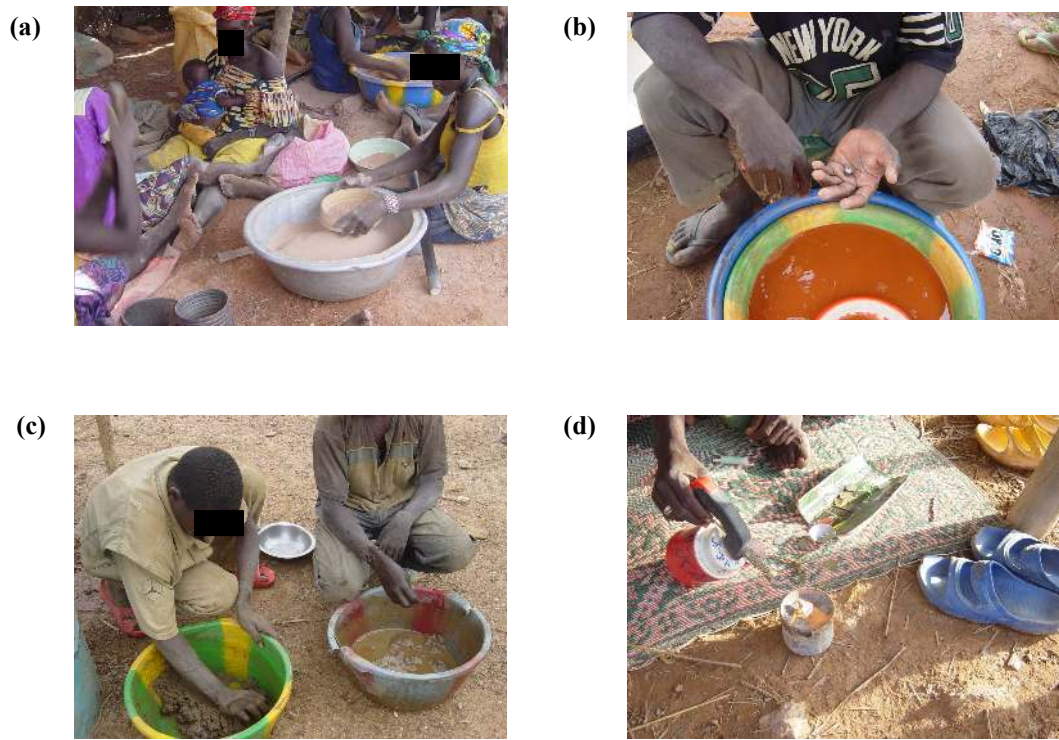
Figure 1. Different steps during the mining process using mercury, on a small-scale gold mine site in Burkina Faso, with (a) ore crushing, (b) and (c) gold-mercury amalgamation, (d) heating of the obtained amalgam.
