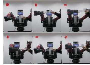
Fig. 6: Subject B performs a co-transporting task with Baxter robot along the direction of red arrows.
