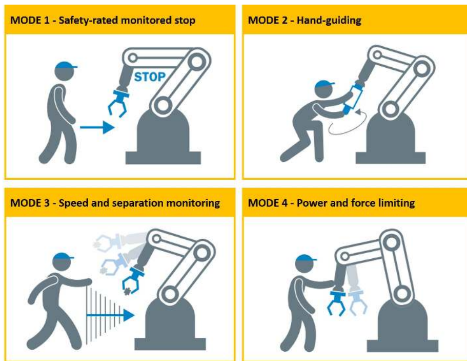
Figure 1: The four forms of collaboration identified by the robot safety standards ISO 10218-1/2 [22, 23] and by the technical specification ISO/TS 15066 [24].
