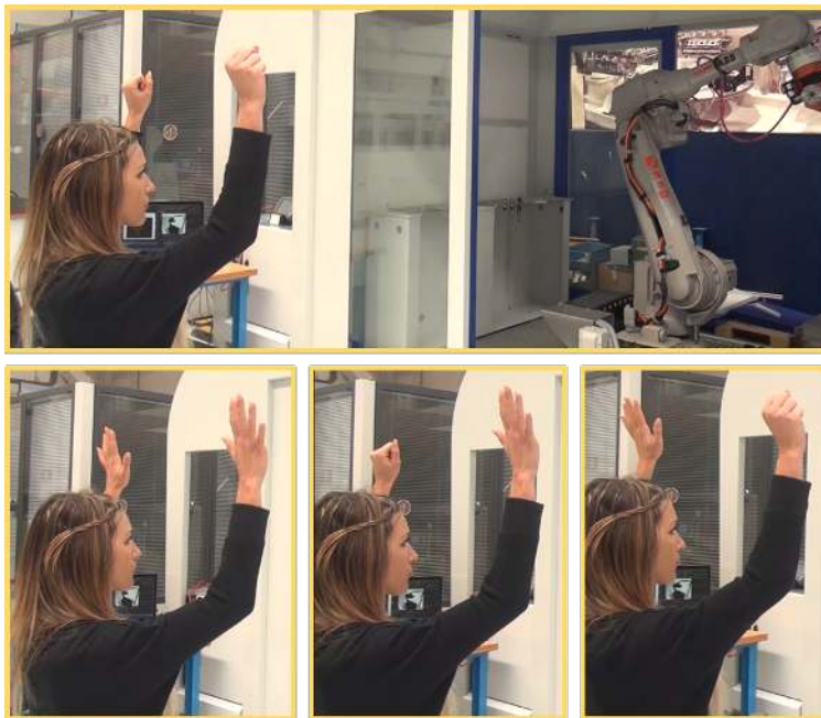
Figure 23: Examples of gestures being performed by a user to command the robot.
