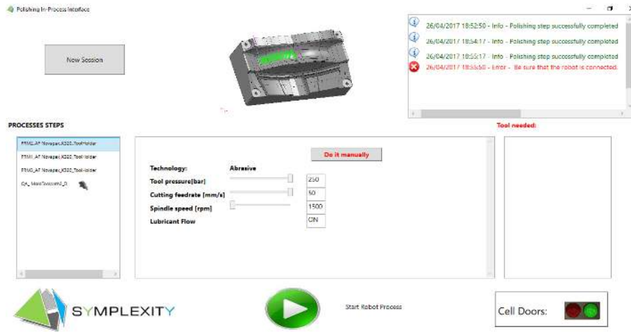
Figure 21: Overview of the in-process interface for the abrasive finishing process.
