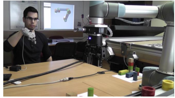
Fig. 3. Human-robot collaborative environment with gesture control interface (left), presentation of a digital twin (centre background), and a physical robot (right).
