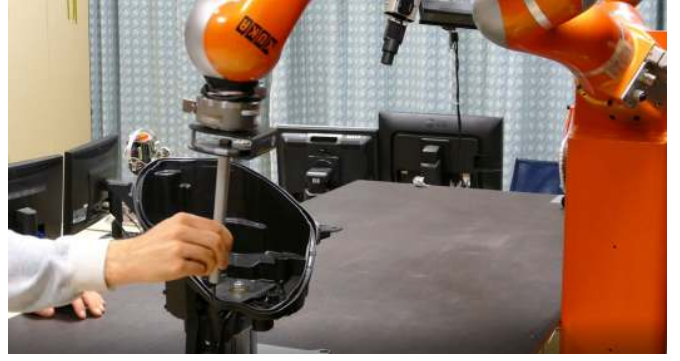
Fig. 3 Learning of a complex trajectory, where the spatial and the velocity part of the trajectory were demonstrated separately.
