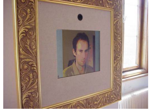
Fig. 1. LCD computer monitor dressed up like a precious painting. The round opening above the picture is for the digital camera lens.
