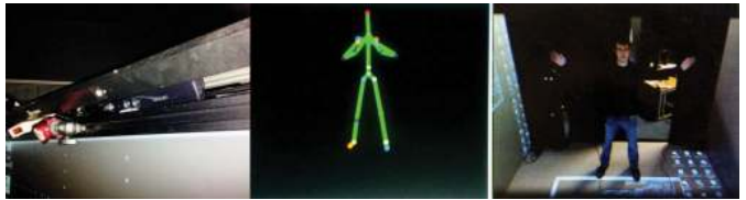
Fig. 1. Kinect tracking in our CAVE system. Left: mounted at a 23° decline in order to maximize the capture volume. Middle: Skeletal tracking. Right: The camera view.
