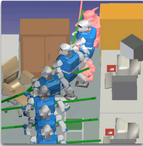
Fig. 10. Generated dynamic path for the heavy object. Collision occurs due to larger effect of task dynamics at the last position (colored red).
