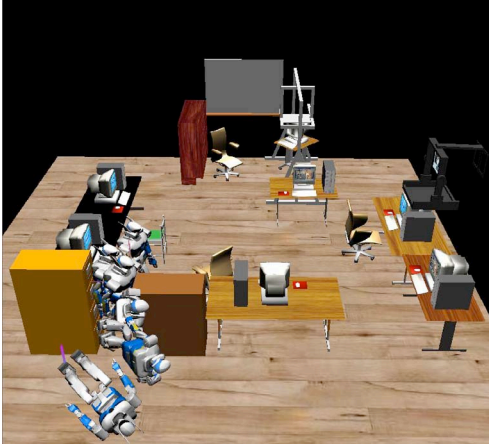
Fig. 6. Collisions generate forces (reaction forces are visualized) and the robot falls (in this example, even if other solutions with higher clearance are possible, we force the robot to enter the narrow passage for path reshaping evaluation purpose).
