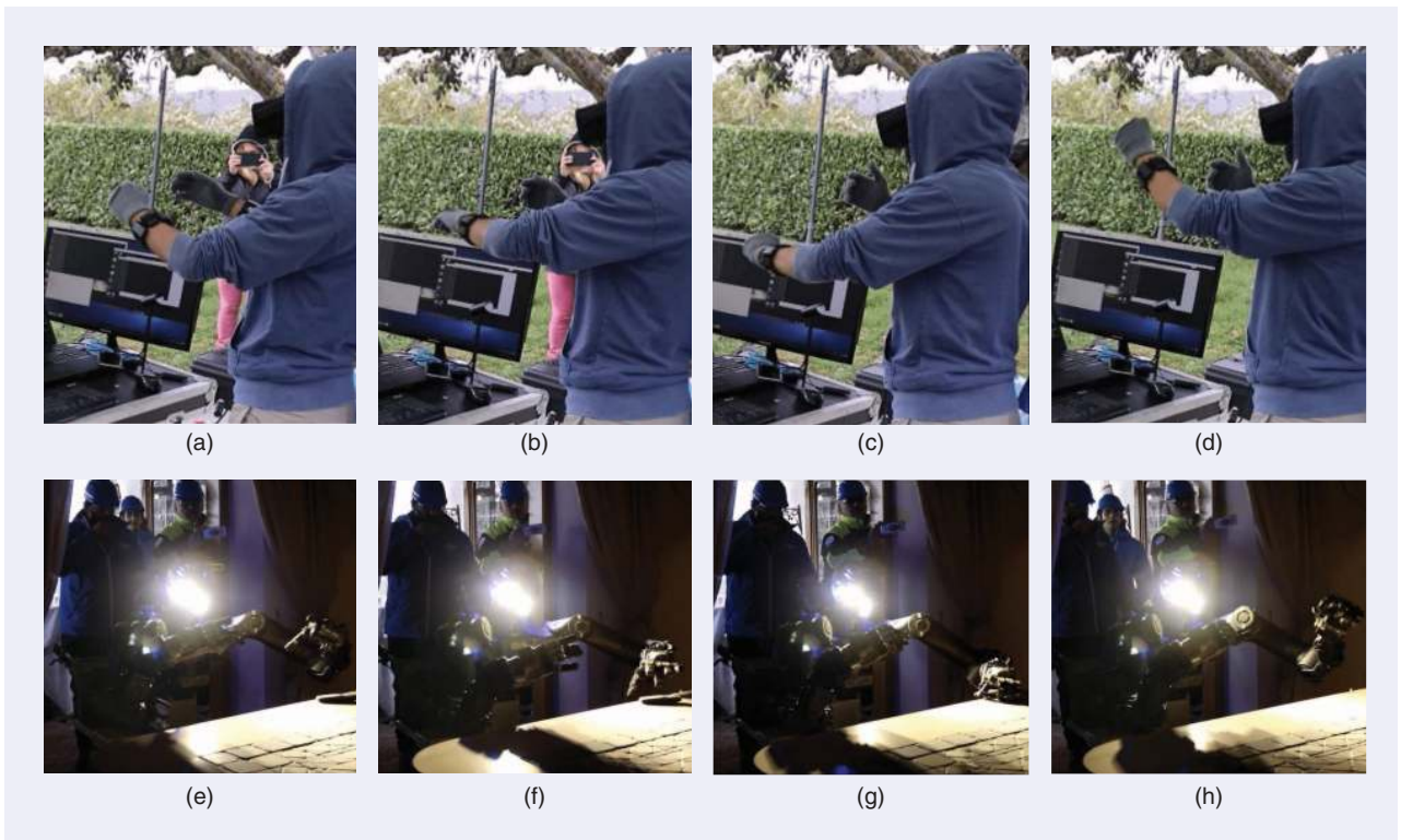
Figure 11. A detail of a manipulation task executed during the field test. (a)–(d) The pilot station is visible, with the operator wearing the Oculus and Myo bracelets. (e)–(h) The robot WALK-MAN executes the commanded actions.
