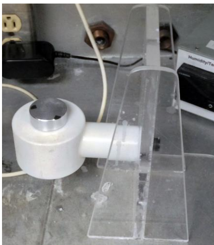
Figure 20: Collector electrode for unaligned fibers
