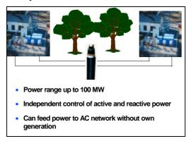
The converter station is designed for a power range of 1-100 MW and for a dc voltage in the 10-100 kV range. One such
