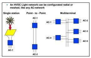
The dc grids can be radial with multi-drop converters, meshed or a combination of both. In other words, they can be configured, changed and expanded in much the same way AC grids are.
