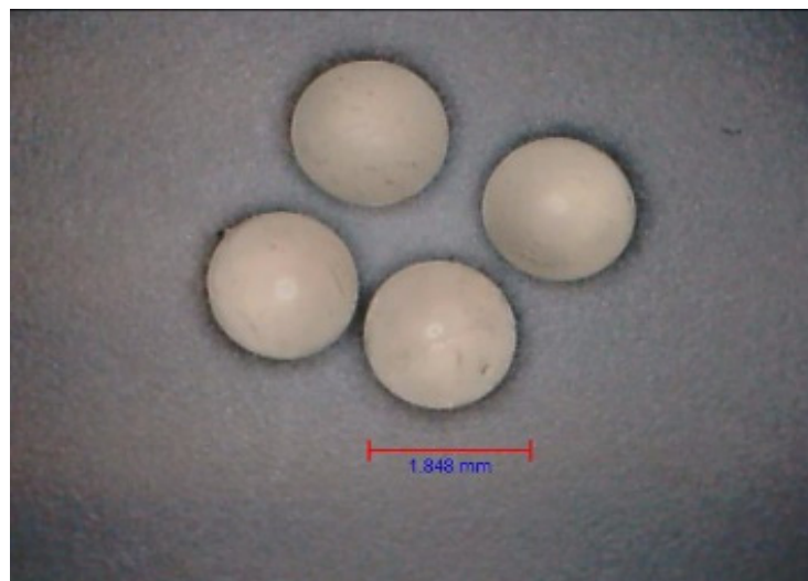
Figure 1. Microscope image of HA-SAL capsules obtained by physical gelation. The head used in the encapsulator had a diameter of 1.5 mm.
