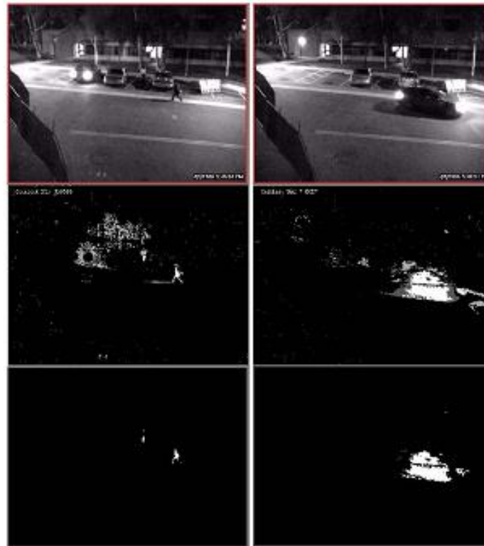
Figure 5. Background Removal at Night. Input (top), Segmentation: shadows as dark gray and highlights as light gray (middle), Final foreground (bottom).
