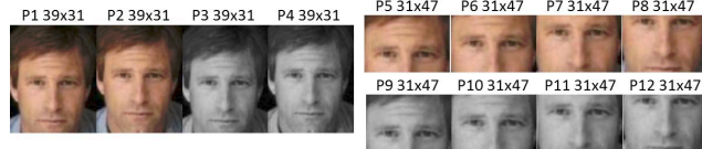
Figure 4: Twelve face regions used in our network. P1 - P4 are global regions covering the whole face, of size 39 \times 31 . P1 and P2 (P3 and P4) differ slightly in the ranges of regions. P5 - P12 are local regions covering different face parts, of size 31 \times 47 . P1, P2, and P5 - P8 are in color. P3, P4, and P9 - P12 are in gray values.
