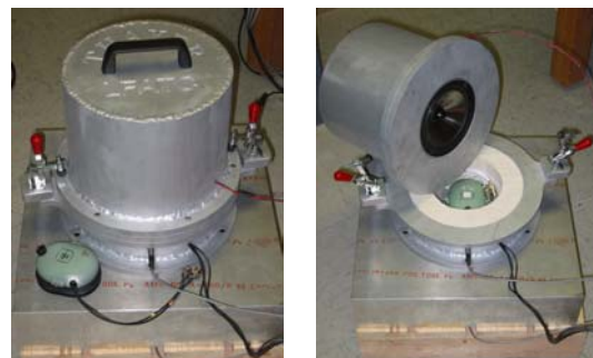
Figure 3: Low Frequency Acoustic Test Cell
