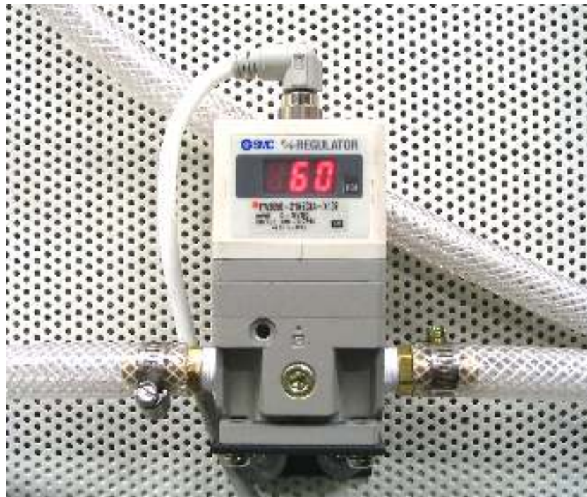
Fig. B.1 Photograph of electro-pneumatic air regulator.
