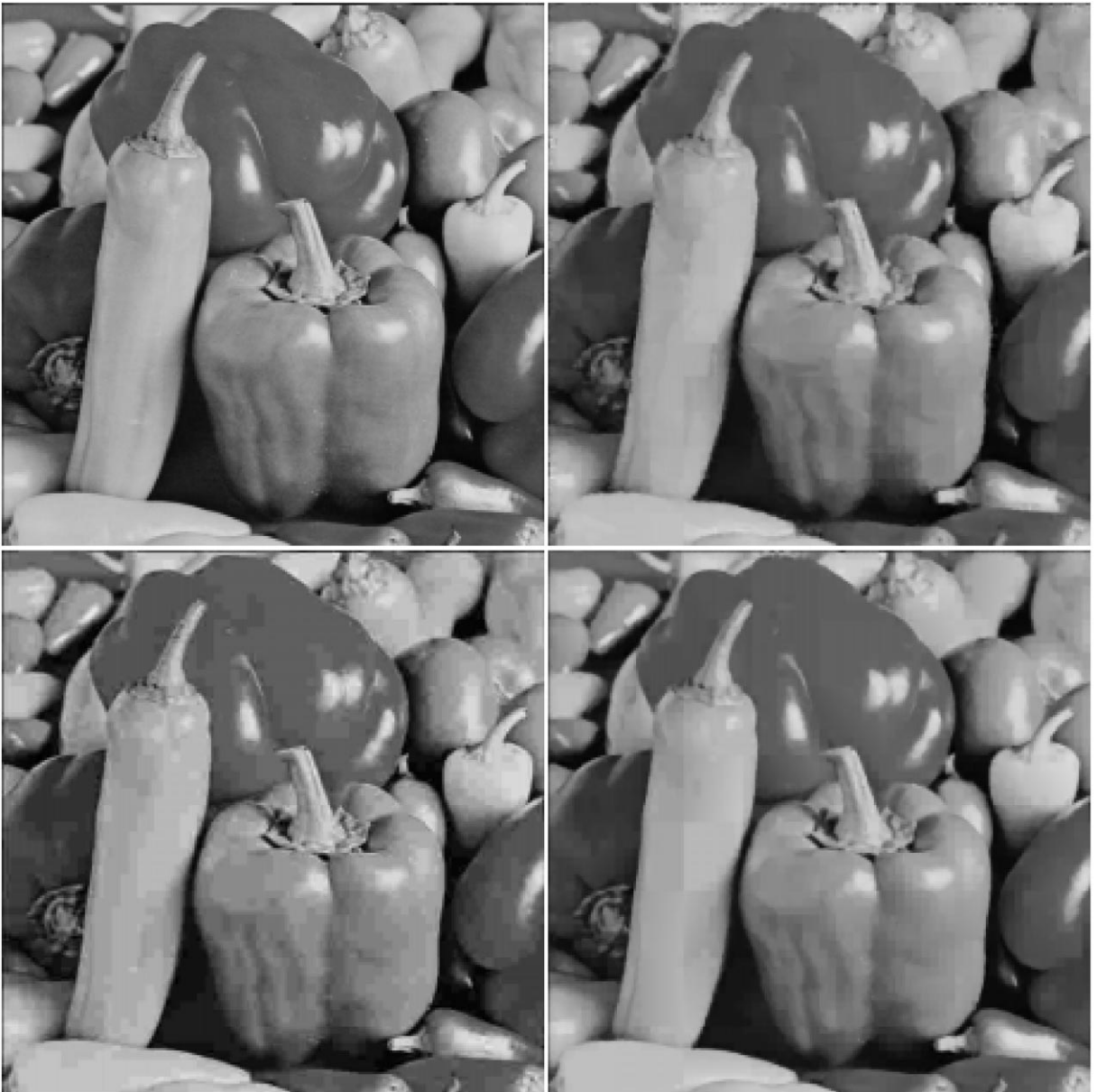
Fig. 6. Original and decoded 'Peppers' images. Upper-left: Original image; Upper-right: Quadtree decoded image, Compression ratio = 34.3, PSNR = 28.7 dB; Lower-left: JPEG decoded image, Compression ratio = 34.0, PSNR = 29.7 dB; Lower-right: Decoded image by the hybrid system, Compression ratio = 35.0, PSNR = 30.5 dB.
