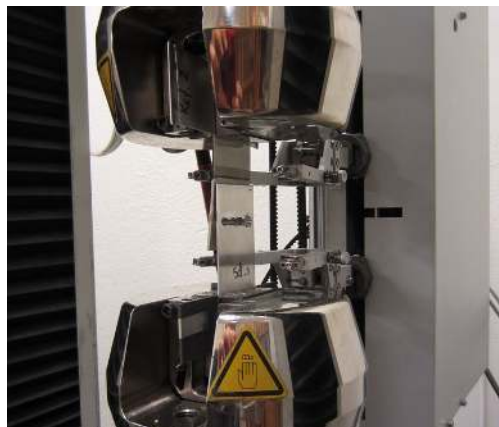
Fig. 20 The photograph showing a specimen in tensile test fixture.
