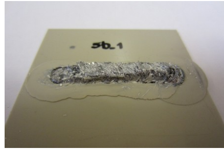
Fig.40 AA5754-PP joint cross section and fracture welded with 1500 rpm, 5 cm/min, 0.5°, CCW
