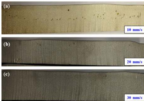
Fig. 5 Effect of the welding speed on the porosity, (a) Test 6, (b) Test 7, and (c) Test 8
