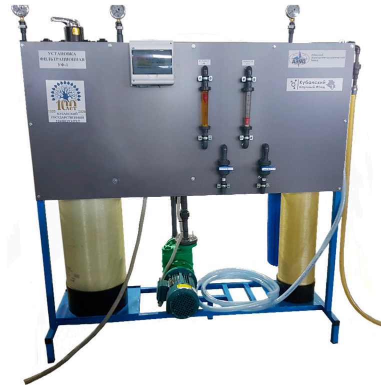
Figure A1. The photo of the filtration module.
