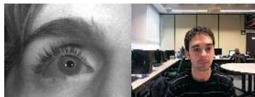
Fig. 1. Images of similar resolution obtained by a high performance eye tracking system (left) in which the optics used and two infrared light-emitting sources permit to obtain a focused image of the eye area. The image obtained by the web cam (right) captures a wider area of the scene.
