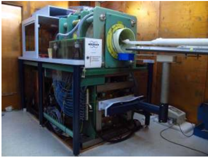
Fig. 1. Photograph of the highly integrated MPI-MRI hybrid system (Bruker BioSpin MRI GmbH, Germany) described and characterized in [20]. The dual-mode main magnetic field generator used in this study features a MRI-modus with B_0 = 0.495 T or G_z = 2.2 T/m in the MPI-modus. In addition, a three-axis MRI gradient, a 2 nd order shim coil set, a TRx radio-frequency MRI coil and a TRx three-axis Drive Field coil are embedded allowing for seamless dual-modal examinations.
