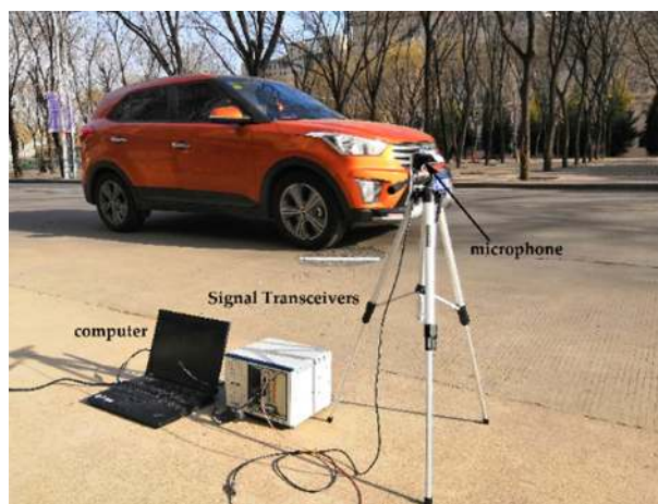
Figure 7. The process of audio recording.
