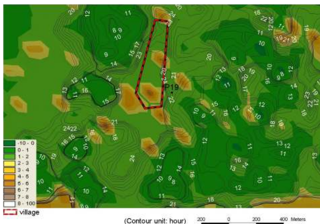
Fig. 14. Topography around P19 with the inundation contours of 20-cm depth advancing with elapsed time (by hour) in Typhoon Sepat.
