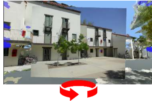
Figure 1: An example interface of orbiting through a set of photos that observe a point-of-interest in a 3D reconstructed scene. This paper investigates different user interfaces for such orbiting-to-photos techniques. Here, blue cameras indicate possible photos to move to, while the currently viewed photo is shown in the center of the screen. The red orbit figure is for illustration only and does not appear in the interfaces.
