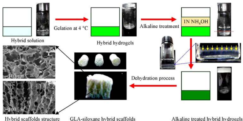
Fig. 4 Schematic diagram showing an experimental procedure for producing anisotropic porous gelatin-silica hybrid polymer scaffolds by ammonium hydroxide treatment. Reproduced from Ref. [68] with permission.
