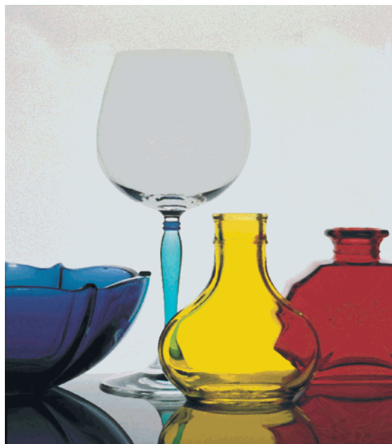
Figure 12. Glassware demonstrating the high quality optical appearance of crystal glass and other types of glasses after being spray coated with colored, sol-gel-derived hybrids.
