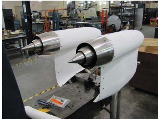
Figure 8. Baseline nozzle installed on the Compact Jet Engine Simulator.
