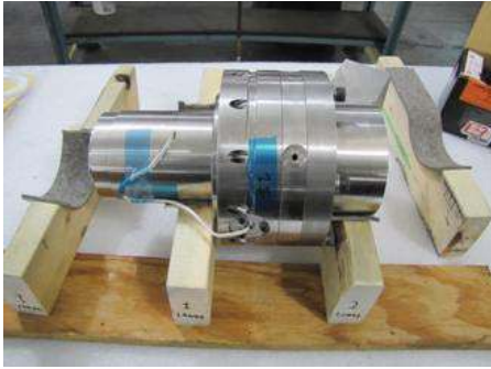
Figure 9. Ultra Compact Combustor for CJES unit. The core air flow enters from the right. Propane combustion is contained in the mid annular section. The fuel and bypass air ports are located circumferentially around the annular combustion section.
