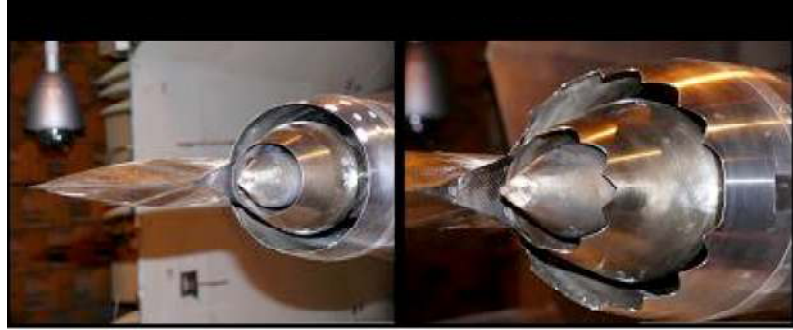
Figure 3: Nozzle configurations, HBPR baseline nozzle with pylon (left) and Chev2 chevron nozzle with pylon (right). Figure from Reference 10.
