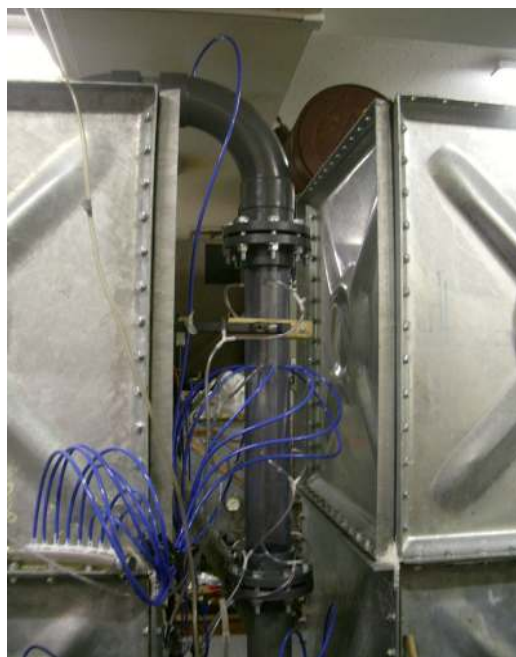
Figure 9: Photograph of siphon rig, showing aerator
