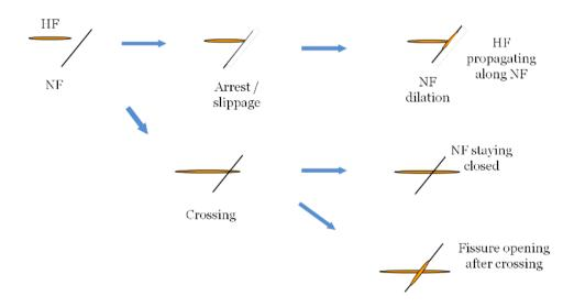
Figure 3. Schematic diagram of possible HF-NF interaction scenarios
