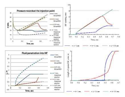
**Figure 11.** Results of numerical experiments with  $\kappa_{IC}$  = 0.32,  $\Sigma_2$  = 0.8,  $\Delta\Sigma$  = 1,  $\beta$  = 90,  $\lambda$  = 0.2 and three values of residual hydraulic opening at the NF permeability (blue: 1 mm; red: 0.1 mm; green: 0.01 mm). Top left: fluid pressure changes at the inlet. Top right: opening of the HF at junction. Bottom left: fluid penetration length along the NF. Bottom right: total length of the mechanically open zone at the NF in meters.
