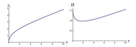
Figure 8. Analytical solution of the dimensionless problem for fluid penetration into NF (34) for dimensionless permeability  $\Psi_h = 1$ , and initial pressure  $\Pi_{00} = 1.5$ . Left plot is the dimensionless fluid front propagation along the NF in time. Right plot is the change of dimensionless pressure at the HF-NF intersection point.
