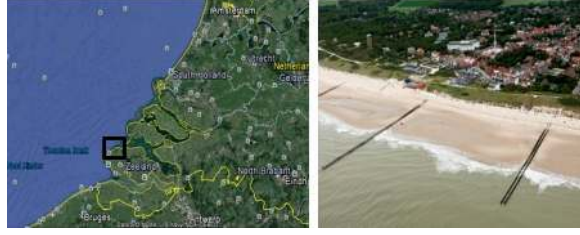
Figure 4.1: Left: The location of a pile groin engineered coast in Zeeland Province, The Netherlands (in the black rectangle, from Google earth); right: the continuous straight shoreline response to PPGs at the coast (source: https://beeldbank.rws.nl , Rijkswaterstaat).
