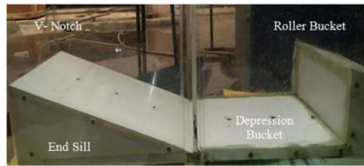
Fig. 1. Modified stilling basin with depression bucket
