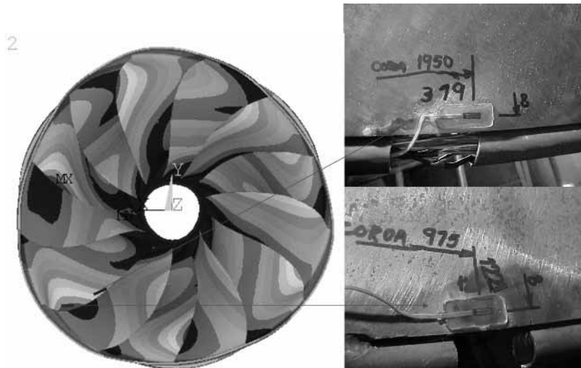
Fig. 9. Strain gages for mode shape investigation.
