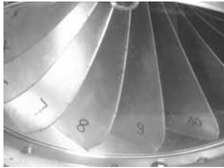
Fig. 3. Flow in the Runner-Best point.
