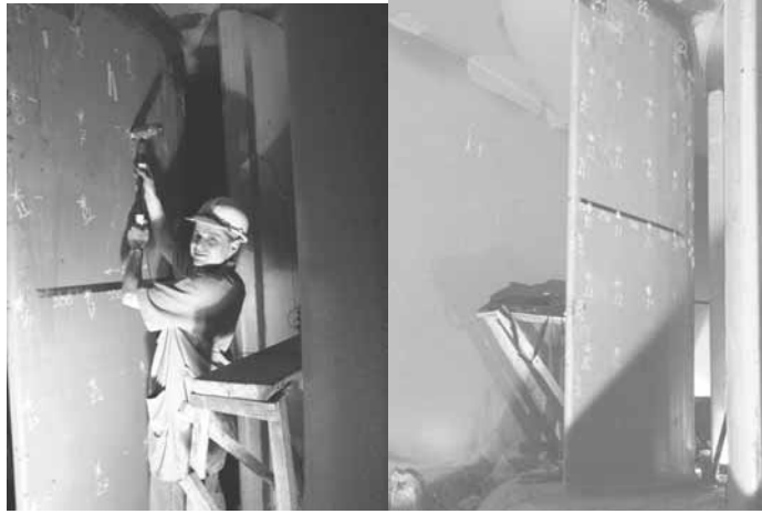
Fig. 12. Mesh and experimental modal analysis technique.
