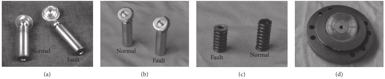
FIGURE 9: Some pictures of the fault elements. (a) Single slipper off fault. (b) Single slipper wear fault. (c) Center spring fault. (d) Swash plate wear fault.
