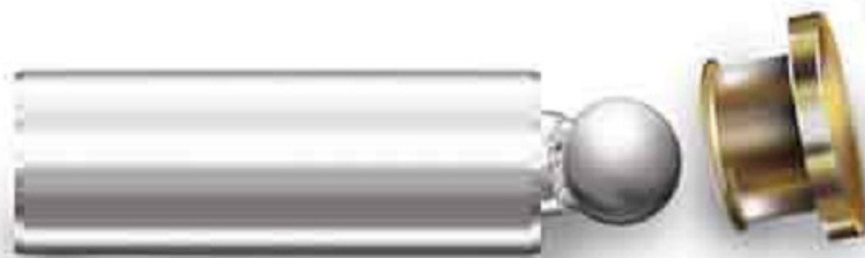
Slika 2. Odvajanje klipa od čahure [10] Figure 2 Separation of the piston from the sleeve bearing [10]
