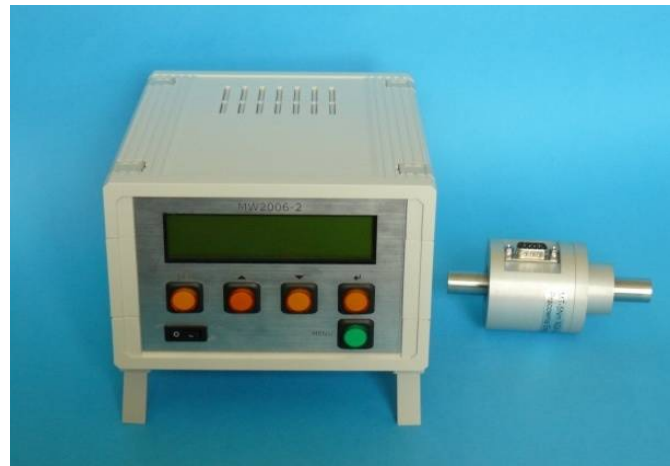
Figure 5. The MT5Nm-N24 torque meter, serial No. 090410 with the Sensor-AT MW2006-2 m, serial No. 090303 [37].
