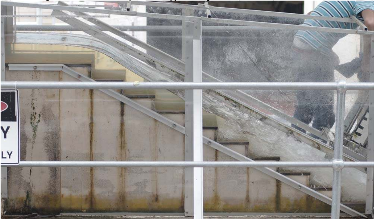
Fig. 2 - Experimental stepped weir
