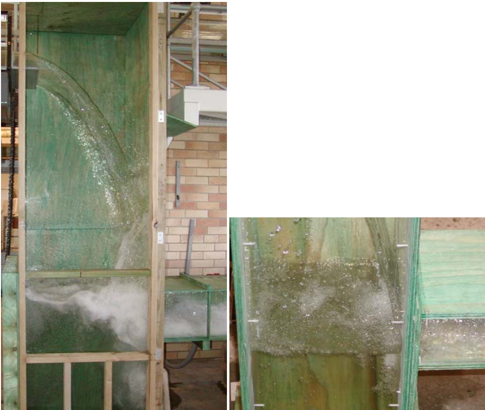
Figure 4 Scale effects in aerated flow situations. Flow direction from left to right on all photographs
