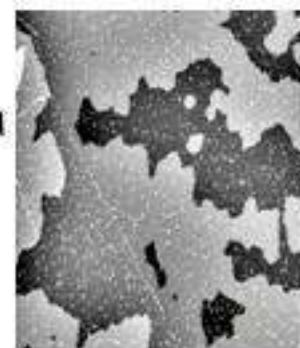
STM picture of Al surface pitted in hydrogen environment
