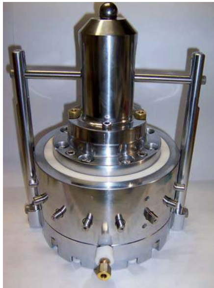
Fig. 1. Oedometer ERT cell used in the investigation.
