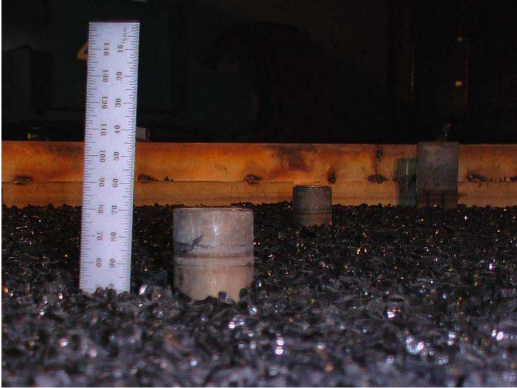
Figure 10 Spectrometer feed through, Medtherm feed through, and TC rake (front to back) in fuel pan.
