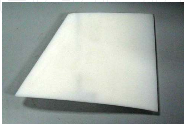
Fig. 19. The photo of the rudder of PETREL
